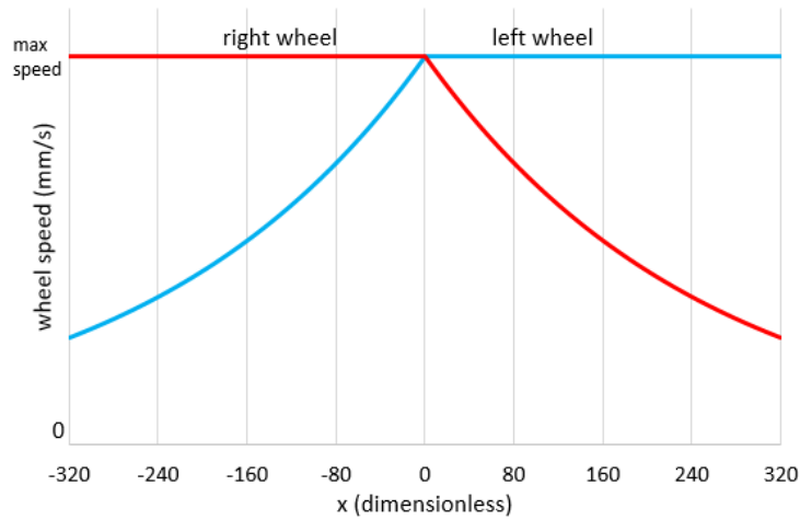
Figure 5.2: Plot of Equation 5.16, with wheel speeds as a function of the combined x value from Equation 5.15. \gamma is set at 0.004, which ensures that the difference between the left and right wheel does not change too dramatically, which would otherwise cause large overshoots.
